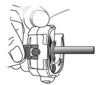
3. Rotate until the pipe is cut.
