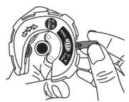
1. Flip handle up and rotate handle to adjust the slide block to the desired size mark.
