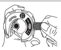
2. Insert pipe into the cutter and rotate as indicated by the arrows on the side of the body.
