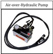
Air Compressor Requirements for use with PESAPA: Regulate the air supply between 100-120 psi at the pump to obtain the rated 10,000 psi hydraulic pressure. Required air flow is 20 CFM to achieve standard pump speeds. Air flow less than 20 CFM will result in slower tool operation.
