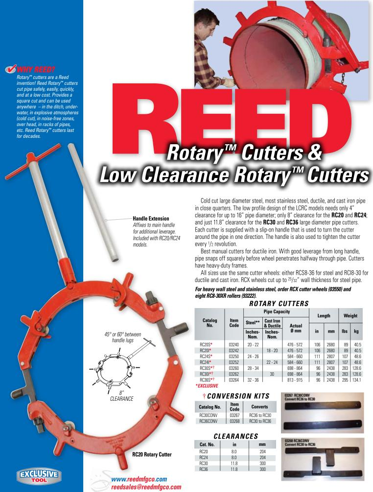
Cold cut large diameter steel, most stainless steel, ductile, and cast iron pipe in close quarters. The low profile design of the LCRC models needs only 4" clearance for up to 16" pipe diameter; only 8" clearance for the RC20 and RC24; and just 11.8" clearance for the **RC30** and **RC36** large diameter pipe cutters. Each cutter is supplied with a slip-on handle that is used to turn the cutter around the pipe in one direction. The handle is also used to tighten the cutter every 1/2 revolution.
